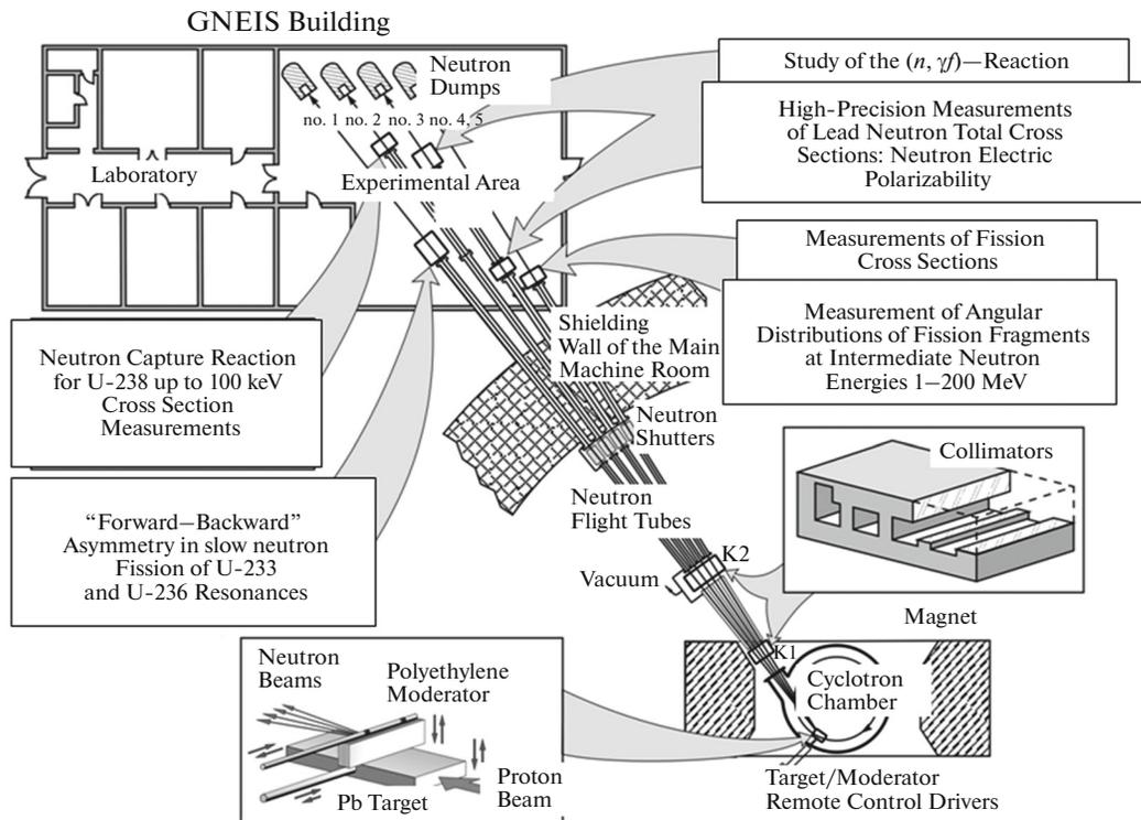
Fig. 1. General layout of the GNEIS facility.
